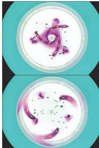
Fig. 4. (at right) The top panel shows near bottom inward circulation, analogous to low-pressure near surface flow, while the bottom panel shows outward circulation near the bottom analogous to the near surface flow for a high-pressure system. (From Ref. 6.)
