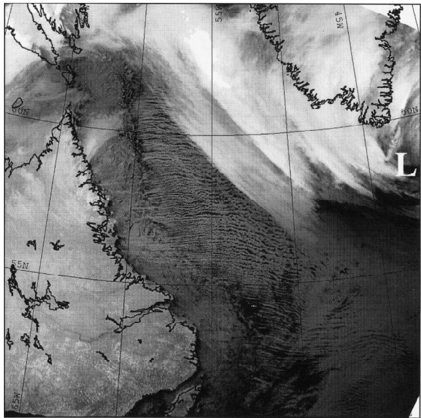
FIG. 2. Infrared advanced very high resolution radiometer image from the NOAA-14 polar orbiter at 1141 UTC on 7 February 1997 showing an extratropical cyclone over the North Atlantic. The location of the low pressure center is indicated by the L. The bright and therefore high clouds to the north of the low pressure center are associated with the system's warm sector. The less bright and therefore shallow clouds to the east of the low, organized into quasi-two-dimensional bands, are associated with the northwesterly flow that results in the advection of cold and dry polar air over the Labrador Sea.
