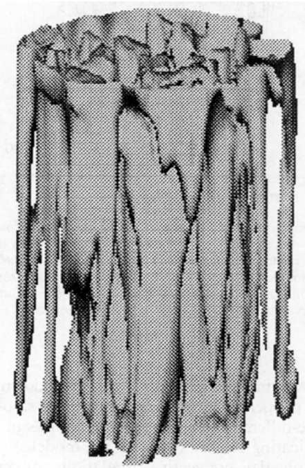
FIG. 5. An isothermal surface from the reference experiment at the end of day 2 capturing the 3D form of the population of sinking plumes.
